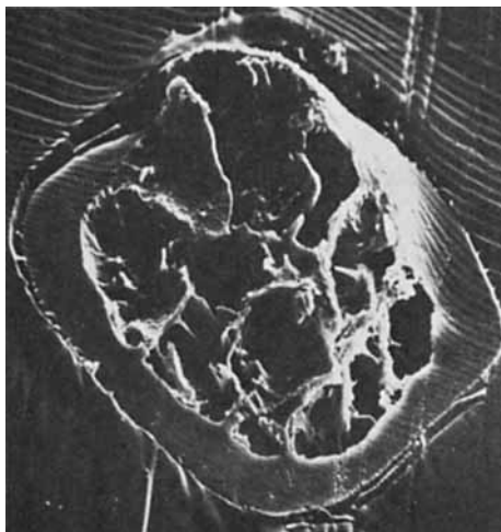
Fig. 9. Scanning electron micrograph of cross section of 63.3% MMA-grafted natural wool (540 \times ).
