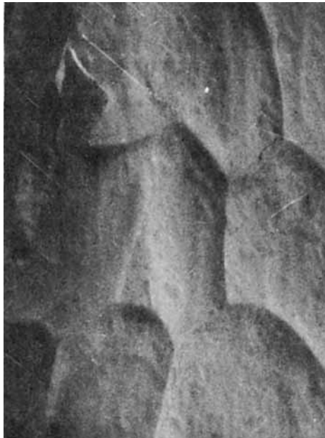
Fig. 5. Scanning electron micrograph of the surface of 35.8% MMA-grafted oxidized wool (1030 \times ).
